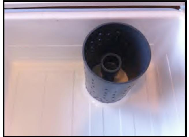
The media guard does not necessarily have to be glued or stuck to the bottom of the growbed - it is a matter of preference, and how likely you think that the media guard might be accidentally moved or dislodged. In the photos above we have used a simple silicon sealant to secure the media guard. If the media guard is not secured then it could make it easier to rotate the media guard at a later date, thus helping to dislodge any roots that might have grown into the guard.
