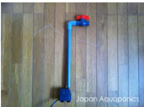
If we are pumping from the Fish Tank up to the Growbeds then there are a couple of things that we would recommend doing. The first is that we need some way of regulating the water flow from the pump and so one very good way of doing this is to incorporate a ball-valve bypass into your system. This bypass is shown here.
